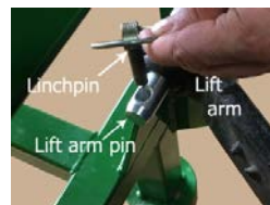
Linchpin above lift arm pin
